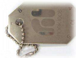
Figure 7 - Internally manufactured welding gauge
