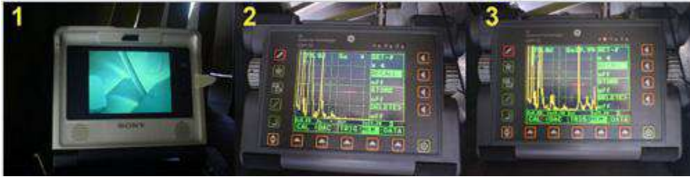
Figure 2 - An example of Ultrasonic Testing (UT) on blade roots of a V2500 IAE aircraft engine .
