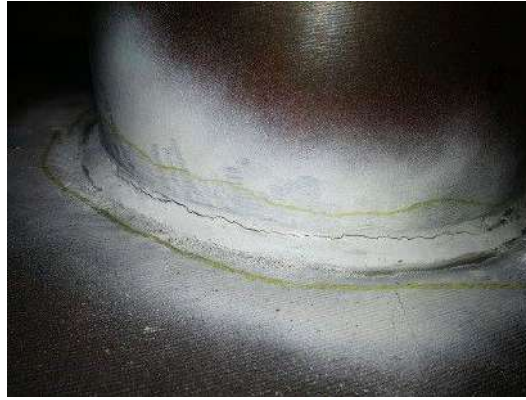
Figure 8 -Representation of the steps performed on the liquid penetrant testing
