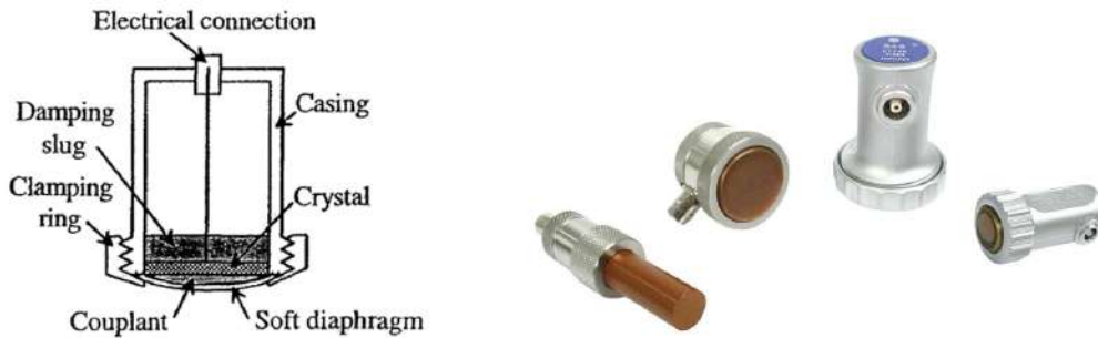
Figure 9 - Straight Beam Contact Transducer
