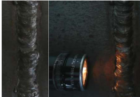
Figure 3 - Localisation of undercut by projecting its shadow
