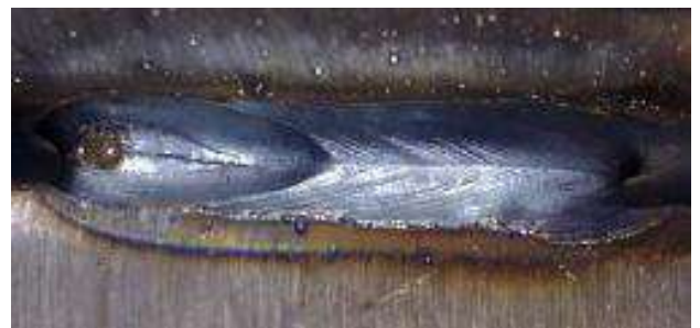
Figure 16 - Cracked spot weld detected during visual pre-weld inspection
